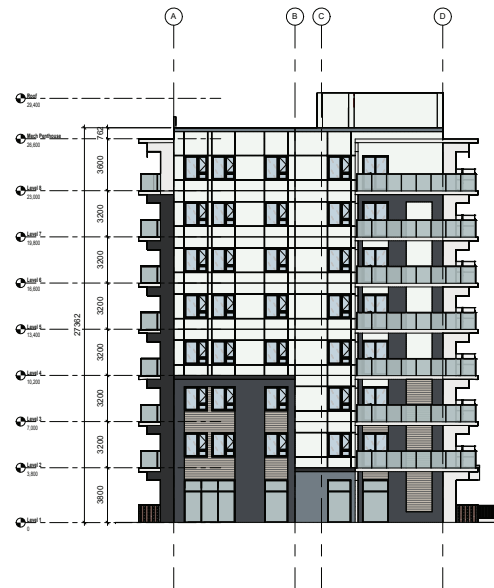
2 BUILDING ELEVATION NORTH A.400 1:200
