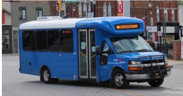
These vehicles are rated for 7-year, 325,000 km life cycle. Detailed mileages by vehicle are not available, however, in seven years from 2015 through 2021, the vehicles will have logged approximately 2.2M kms in total, or approximately 350,000 kms per vehicle.
