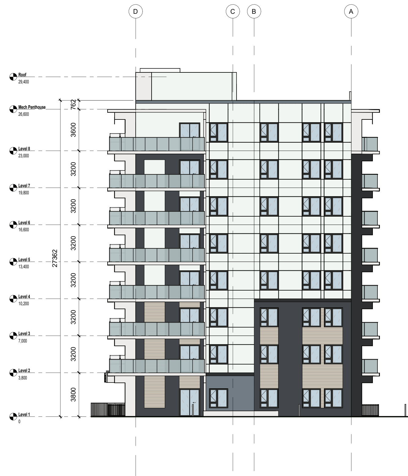
1 BUILDING ELEVATION - SOUTH A.400. 1:200
