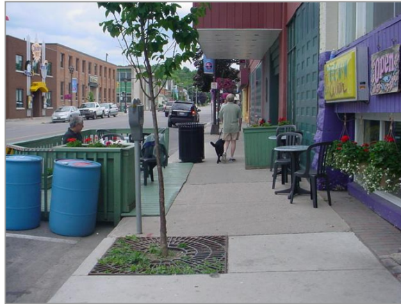
Protrusions force pedestrians to zigzag through obstructions in the path adjacent to a sidewalk
