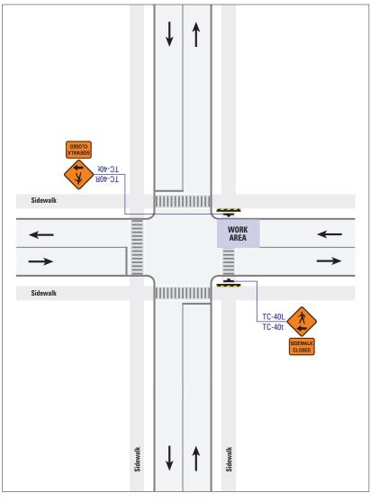
i) Supplementary layout. This layout shows pedestrian signage only and shall be used in conjunction with other appropriate layouts. ii) See TS-21, TS-22, and TI-9 for required signage for vehicle Detour. For further detail on Work Zone components, see Table B (Short/Long, pg. 6). TI-16 Pedestrian Detour: Crosswalk Closure lobile Operations Intermittent Very Short Duration Short Duration Long Duration
