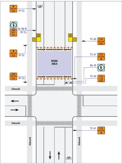
i) Supplementary layout. This layout shows cyclist signage only and shall be used in conjunction with other appropriate layouts. ii) See TS-21 & TS-22 for required signage for vehicle Detour. iii) Ramps must be AODA-compliant. For further detail on Work Zone components, see Table B (Short/Long, pg. 6). TI-19 Bicycle Lane Closed: Dismount and Walk Mobile Operations Intermittent Very Short Duration Short Duration Long Duration 75
